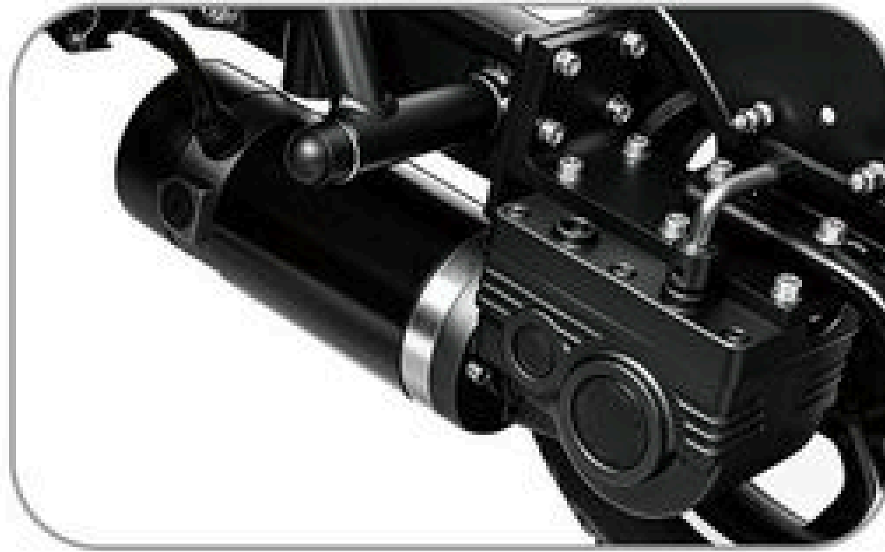
1000W蜗轮蜗杆电机，动力十足 1000W worm gear & worm drive motor full of power
