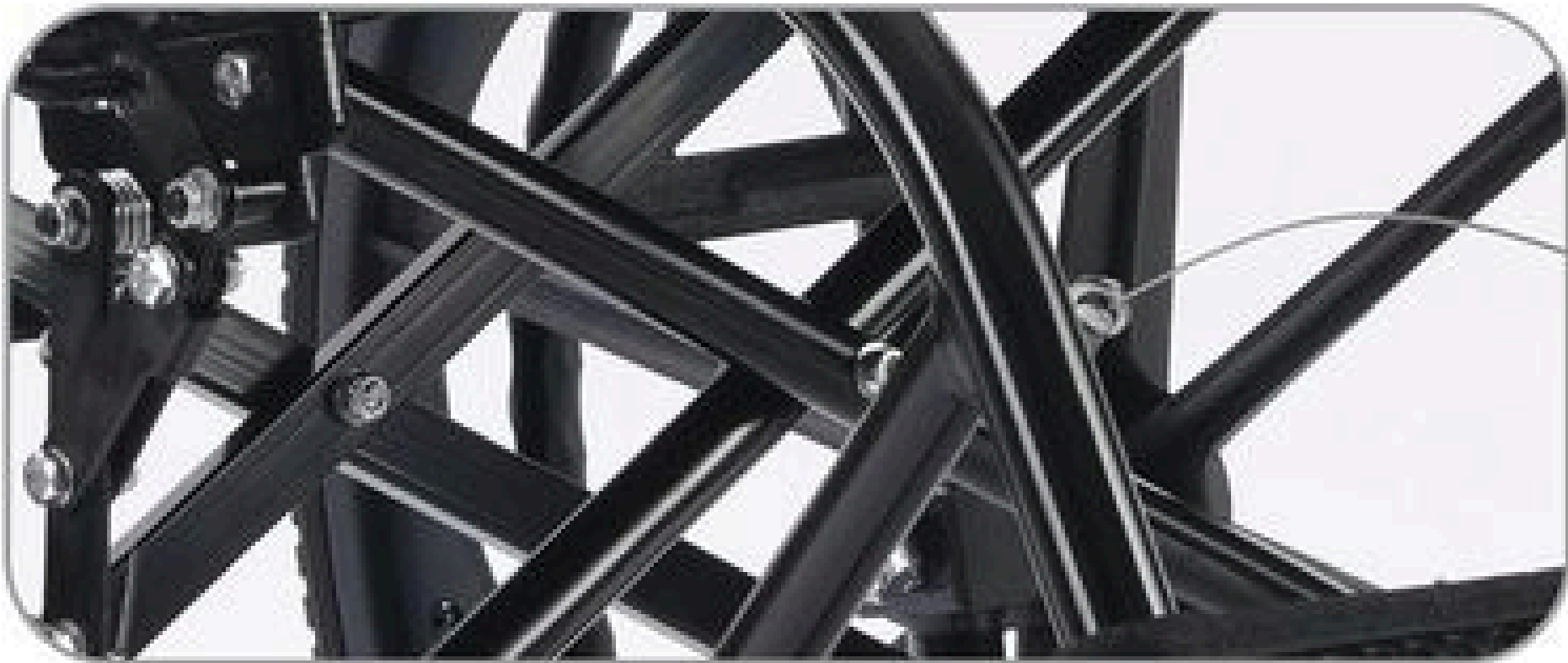
双X中叉设计 Dual x-shaped mid-frame structure
