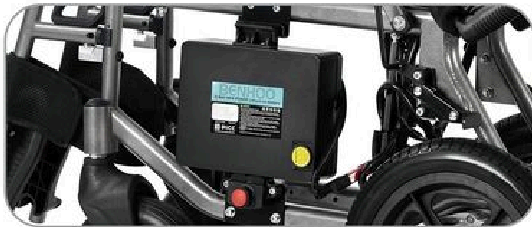
快拆式锂电池 Quick-release lithium battery
